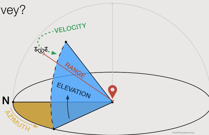
Radar is only as good as the data it conveys to the user. If the radar receives incomplete, unclear, non-actionable data, the available system data is just a dot on a map that conveys nothing but anxiety. To understand what a radar can, and should, convey, it is important to understand the following four data dimensions of radar:
