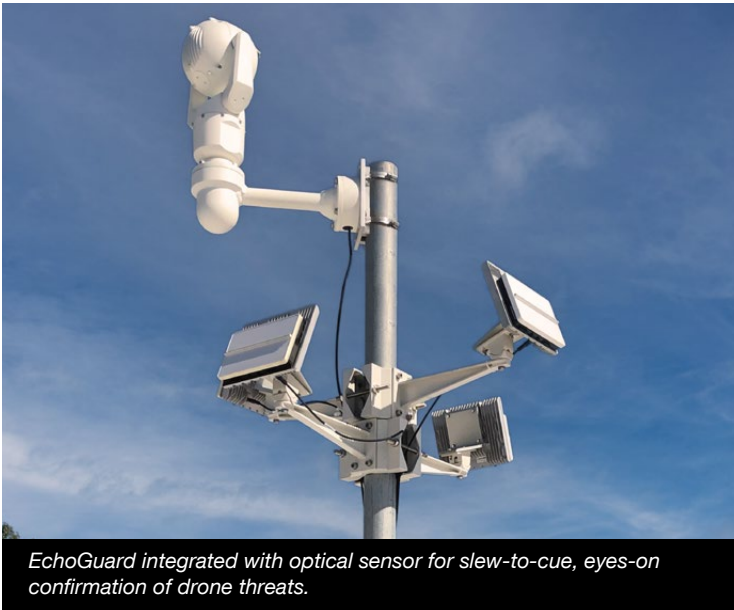
Improving situational awareness with single pop-up radars for drone detection and tracking at high-profile event.
