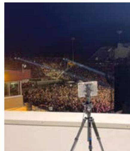
EchoGuard deployed for drone detection at mass gathering.
