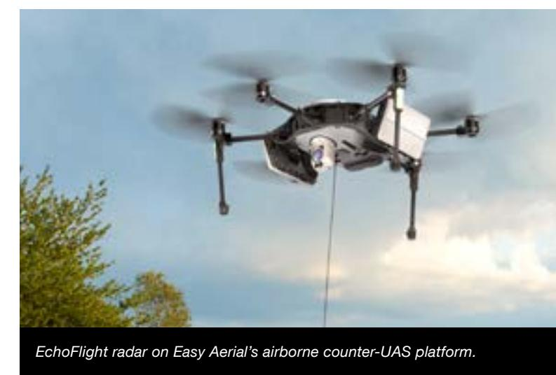
EchoFlight radar on Easy Aerial's airborne counter-UAS platform.
