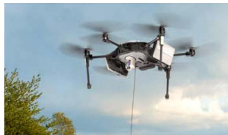
EchoFlight radar on Easy Aerial's airborne counter-UAS platform.
