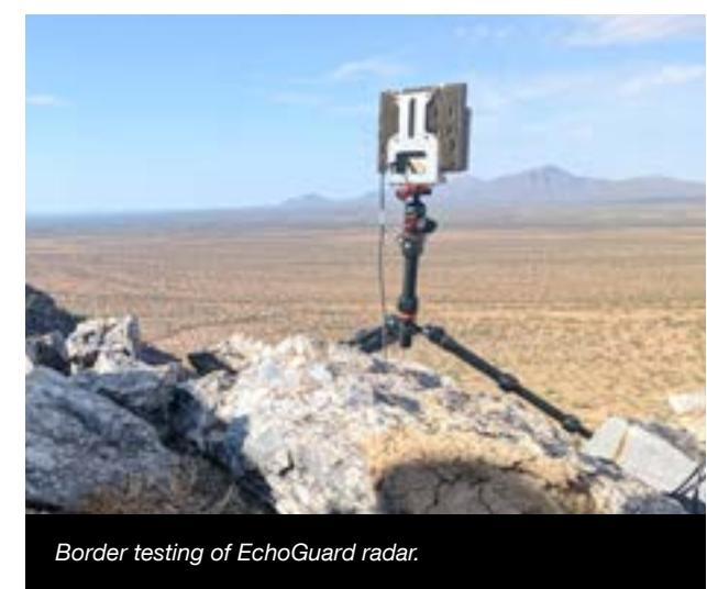
Border testing of EchoGuard radar.
