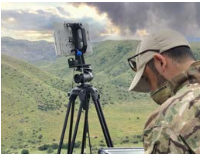
EchoGuard radars deployed for discrete surveillance.
