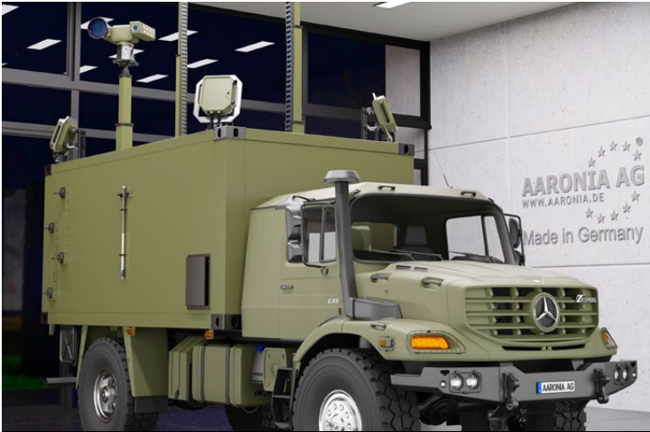
EchoShield radars configured for on-the-move (OTM) application.
