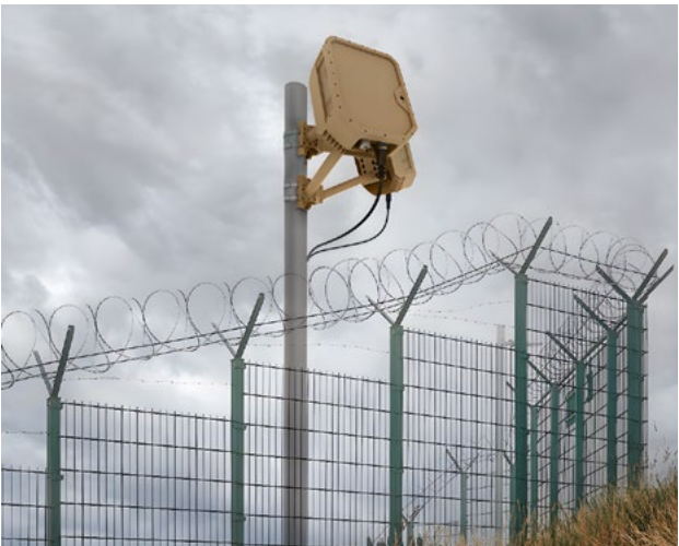
Extended perimeter intrusion detection at high security site using EchoShield.
