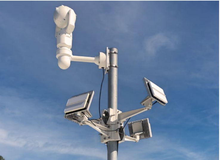
EchoGuard integrated with optical sensor for slew-to-cue, eyes-on confirmation of drone threats.
