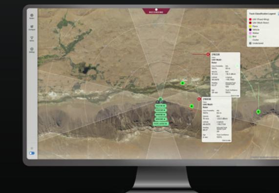
EchoWare combines advanced MESA capabilities with powerful off-radar software to deliver an abstraction layer that seamlessly integrates multiple (n) Echodyne radars into a single radar instance.
