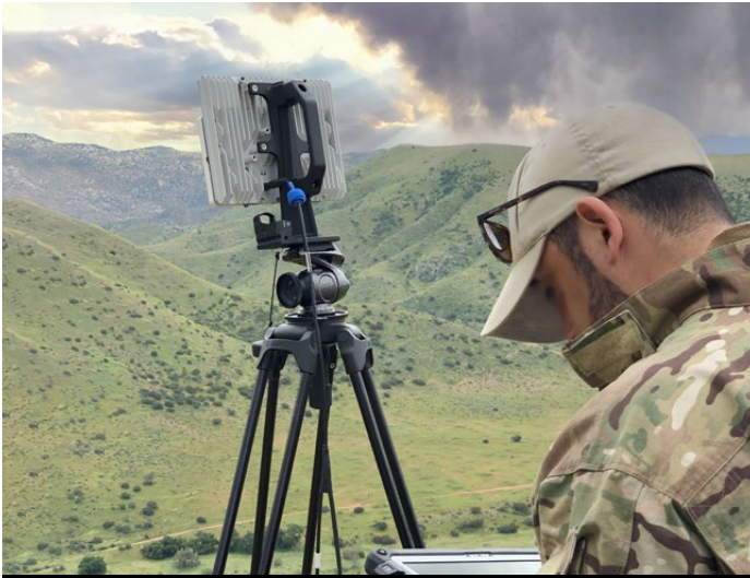
EchoGuard radars deployed for discrete surveillance.
