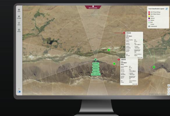
EchoWare combines advanced MESA capabilities with powerful off-radar software to deliver an abstraction layer that seamlessly integrates multiple (n) Echodyne radars into a single radar instance.
