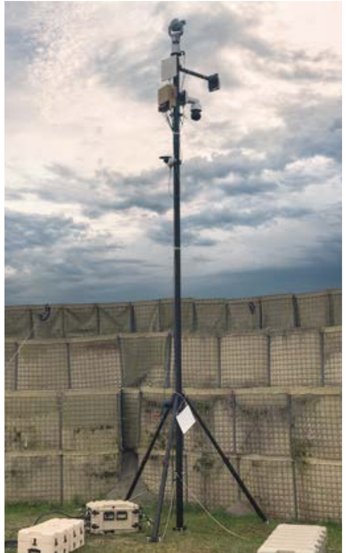
EchoGuard radars are the baseline of the U.S. Army's Security and Surveillance (SSS) program.
