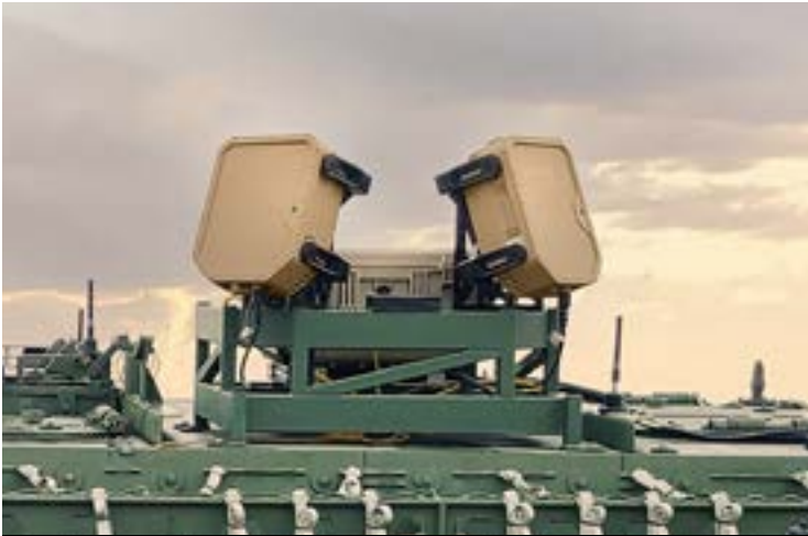
EchoShield radars configured for on-the-move (OTM) application.
