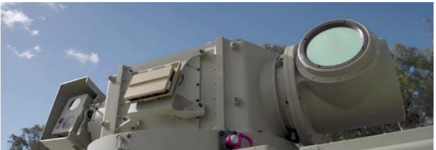
EchoGuard as targeting sensor on EOS Titanis Counter-UAS system.
