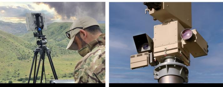
EchoGuard radars deployed for discrete surveillance.
