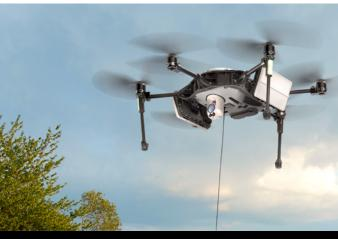
EchoFlight radar on Easy Aerial's airborne counter-UAS platform.
